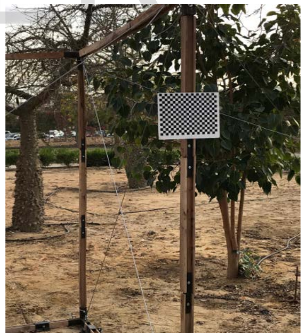
Fig. 15. Monitoring target attached to tested structure
